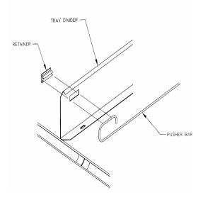
Figure 5.3 Pusher Bar Installation
