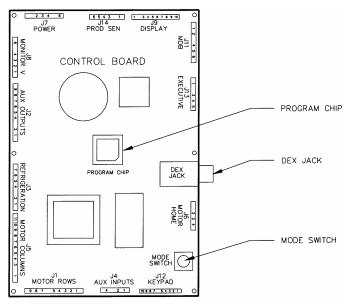
**Figure 3.1 Control Board Components**
