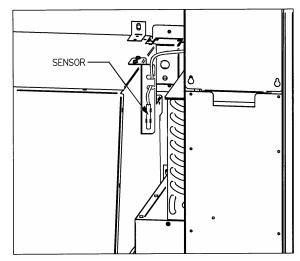
Figure 8.3 Temperature Sensor
