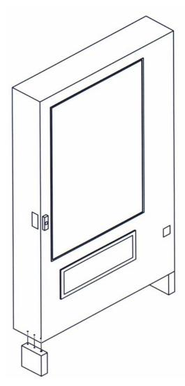
Figure 4.2 False Leg Installation
