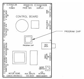
Figure 8.1 Replacing Program Chip
