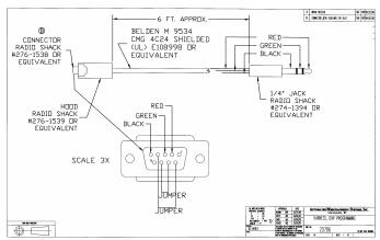
Figure 8.4 Harness, Chip Programming
