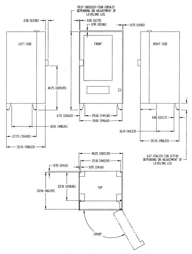
Figure 1.2 AMS 39-VRM Cabinet Dimensions (Inches[mm])
