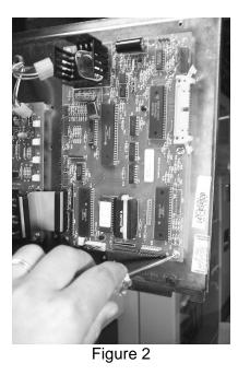
Locate the VMC in the kit. This will mount directly onto the existing standoffs using the same mounting holes. See Figure 3 for correct orientation (board is labeled 147/148 BOTTOM to indicate the proper direction). Use seven of the original screws for mounting.
