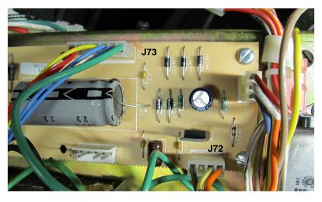
Install cable, 11-0223-21, as a jumper between connectors J72 and J73.
