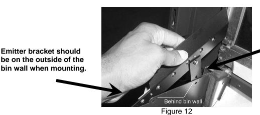
Make sure the extension bracket is between the bin wall and brace.
