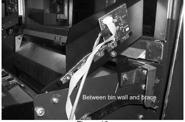
Make sure the extension L-bracket is between the bin wall and brace.
