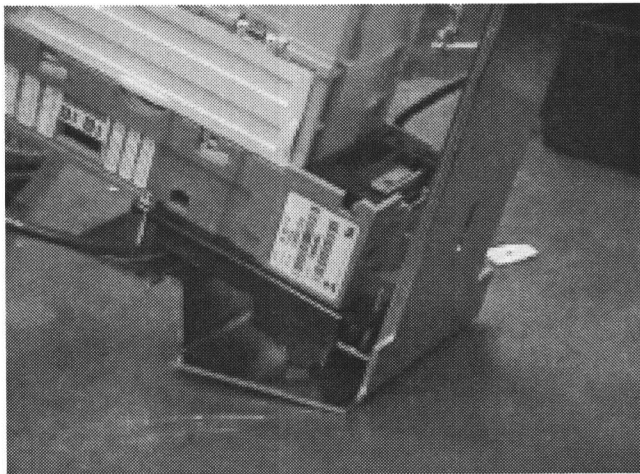
Figure 4 Mounting the validator to hte slider bracket
