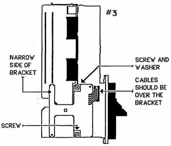
ROTATE MOUNTING BRACKET AS SHOWN INSTALL WASHER AND SCREW AT TOP HOLE AND SCREW IN LOWER HOLE.
