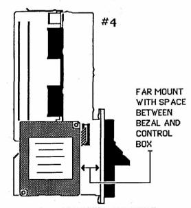
PUT COVER ONTO BRACKET, BE SURE NOT TO PINCH THE WIRES. IT SHOULD LOOK LIKE #4 WHEN DONE.
